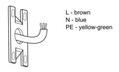
The L, N, PE wires should be connected properly to the power supply wires, and the connection should be sealed to prevent flooding, for example: using a cable gland, an electrical terminal block in an IP box filled with insulating resin, or through a 3-pole connector with a minimum IP65 rating.
