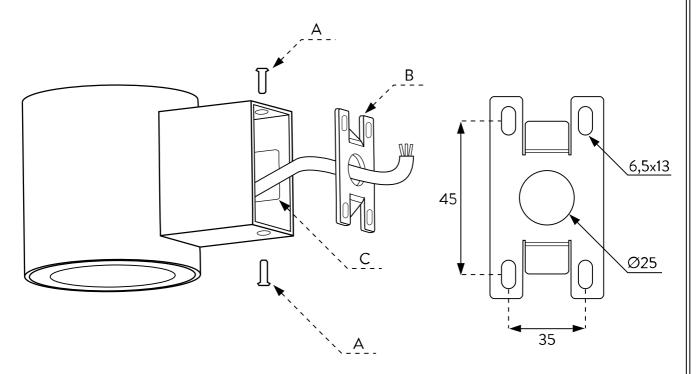
Unscrew screws A and remove bracket B. Check the compatibility of the planned installation with sticker C (light direction up/down). Secure bracket B to the surface using expansion plugs, making sure to pass the power cable through the central hole. Slide the fixture onto bracket B and secure it with screws A.
