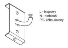
The L, N, PE wires should be connected properly to the power supply wires, and the connection should be sealed to prevent flooding, for example: using a cable gland, an electrical terminal block in an IP box filled with insulating resin, or through a 3-pole connector with a minimum IP65 rating.
