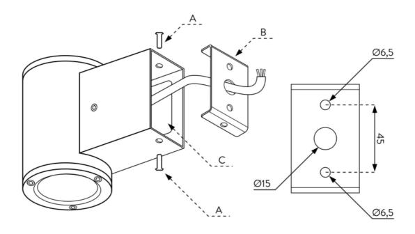
Unscrew screws A and remove bracket B. Check the compatibility of the planned installation with sticker C (light direction up/down). Secure bracket B to the surface using expansion plugs, making sure to pass the power cable through the central hole. Slide the fixture onto bracket B and secure it with screws A.
