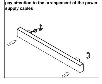
Place the luminaire on the mounting holders,
