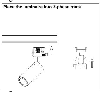
Lock the luminaire in the 3-phase track
