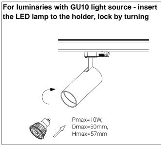
Select the appropriate phase with the knob on adap-ter (pos. 1, 2, 3). Pos. 0 - power supply disconnected
