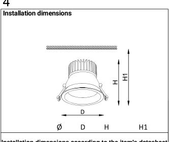
Installation dimensions according to the item's datasheet
