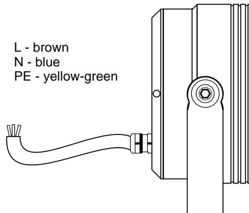
The L, N, PE wires should be connected properly to the power supply wires, and the connection should be sealed to prevent flooding, for example: using a cable gland, an electrical terminal block in an IP box filled with insulating resin, or through a 3-pole connector with a minimum IP65 rating.
