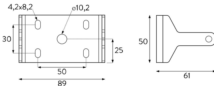
1. Mount bracket B on the surface using expansion plugs.
