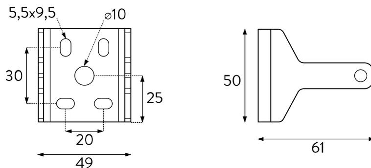
1. Mount bracket B on the surface using expansion plugs.
