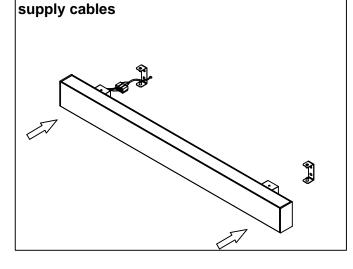
Place the luminaire on the mounting holders,
